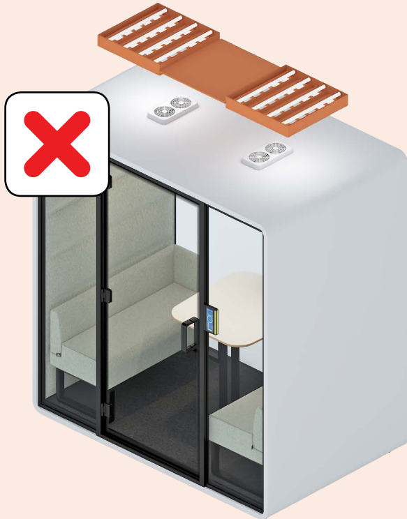
Pod placed under heat sources
